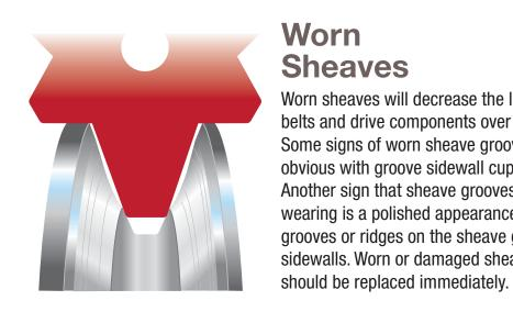
Worn **Sheave Gauge Sheaves** Gates offers sheave gauges that aid in determining the correct belt or sheave cross section. Sheave Worn sheaves will decrease the life of belts and drive components over time. groove wear. Some signs of worn sheave grooves are obvious with groove sidewall cupping. Another sign that sheave grooves are wearing is a polished appearance with grooves or ridges on the sheave groove sidewalls. Worn or damaged sheaves
