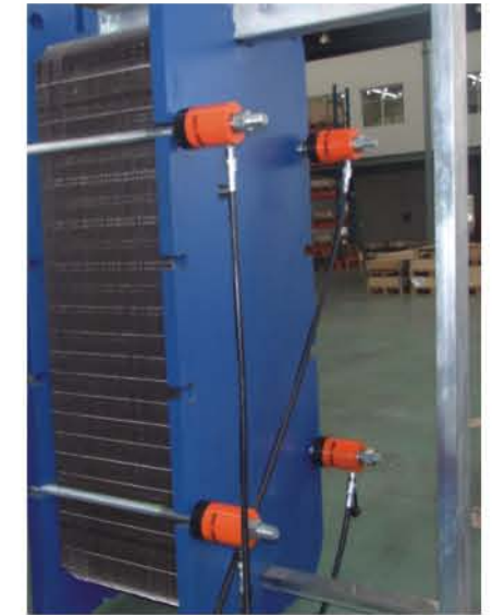
4 EAGLE PRO ESH-306 pulling threaded bar in a the largest heat exchanger in SONDEX's factory in Ningbo China.
